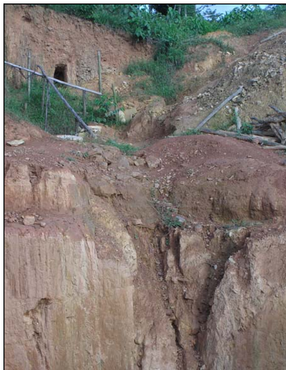
Figure 15.1a. Photo of the Tindika artisanal site illustrating the auriferous quartz vein that is being exploited.
